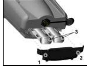
*In the event of nonprolonged use, remove the alkaline batteries from the detector.*
