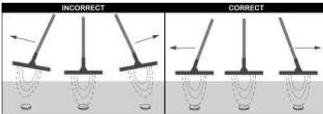
To pinpoint a target, use quick crossed sweeps, with the coil over the target taking note of where the strongest audio signal is received.
