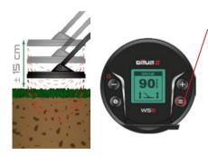
From the Grab menu, you can calibrate the ground effect at any time by holding the key down while you pump the coil on the soil until the ground audio signal is attenuated and the value is stabilized.
