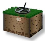
Position the coil barely off the ground and to the side of the target. Press • to calibrate the threshold.
