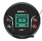
, Access to PINPOINT screen Press 2 seconds lacktriangle, then update the detecting threshold with lacktriangle.
