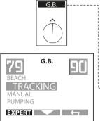
The Ground Notch complements the ground balance settings: it enables a "window" of ground value to be rejected rather than rejecting all the ground values below the setting. You can for example adjust the ground balance on the value of the prospected ground (eg: 78), then reject the false signals due to hot-rocks by adjusting the NOTCH GROUND between 83-90 only, thus you will not reject the ground value from 78 to 83.
