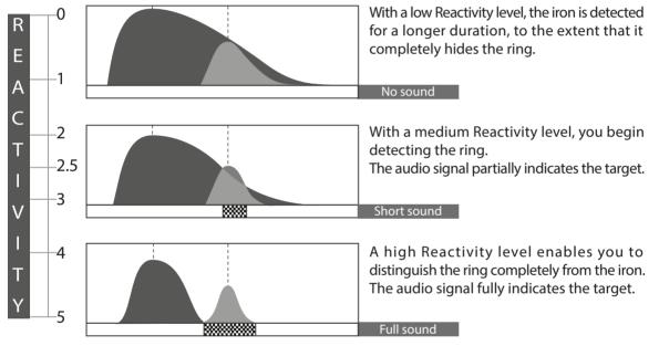
In terms of pure performance, the greatest detection ranges are obtained with low reactivity levels. However, you will find more targets and will detect deeper on mineralised ground with medium or high reactivity levels.
